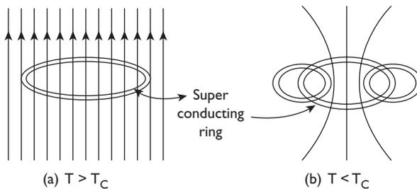
This is due to the diamagnetic property (i.e.,) the magnetic flux inside the ring will be trapped in it and hence the current persists.
