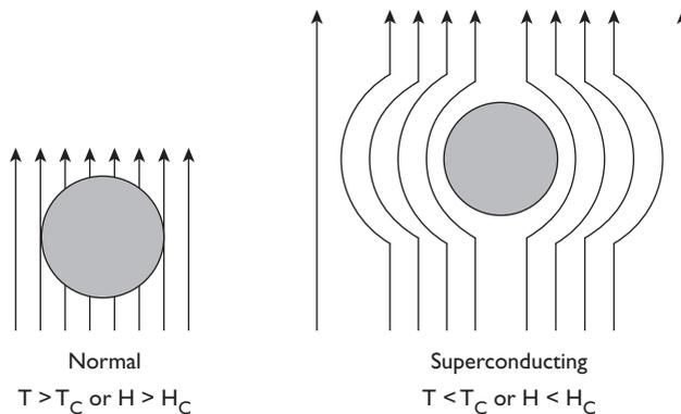
Now when the material is cooled below its transition temperature when ( $T \leq T_C$ ) then the magnetic lines of forces are expelled or ejected out from the material as shown in Figure 4.3(b).
