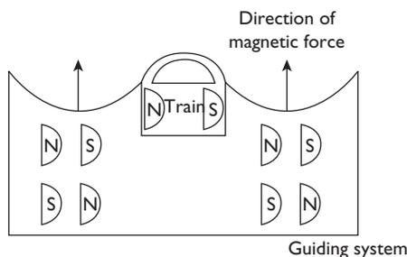
Initially when the train starts, they slide on the rails. Now, when the train moves faster, the superconducting magnets on each side of the train will induce a current in the '8' shaped coils kept in the guidance system.
