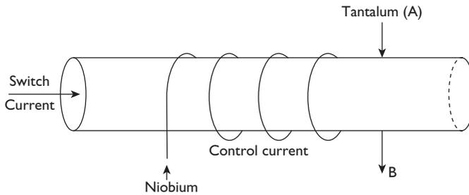
Now, at operating temperature, the magnetic field produced by the material 'B' may exceed the critical field of 'A.' Hence the material 'A' becomes a normal conductor because the critical field of 'A' is less than the critical field of 'B.' Also 'B' will not become the normal conductor at the critical field of A because  $H_{C_B} > H_{C_A}$ .
