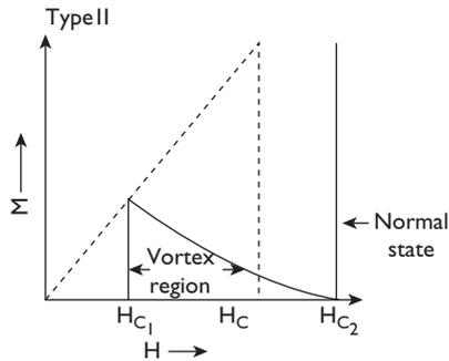
The material which loses its superconducting property gradually due to the increase in magnetic field is called type II superconductors.
