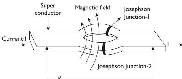
Therefore, SQUIDS are used to detect the variation in very minute magnetic signals. They are used as storage devices for magnetic flux.
