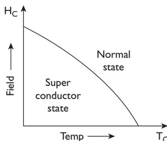
The field required to destroy the superconducting property is called critical magnetic field ( $H_C$ ). It is given as
